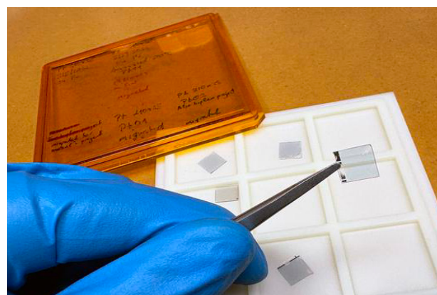
A new platinum-based hydrogen sensor has been recently developed. Picture credit: Chalmers University of Technology | Mia Halleröd
