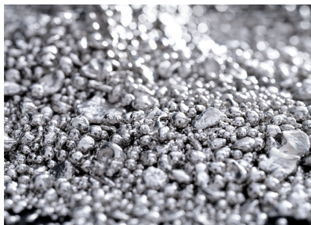
Inoveo Platinum has been developed to be 40% harder than standard platinum alloys. Picture credit: PGI
