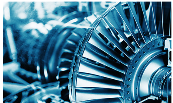
Turbine blades used in aircraft jet engines can be platinum plated to create high-temperature resistance and improve durability
