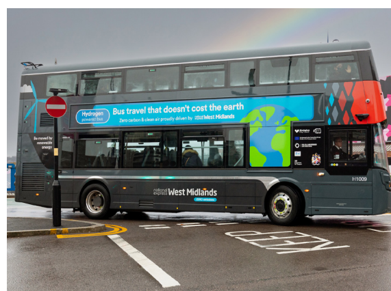
Hydrogen-powered fuel cell buses are being deployed across the UK's West Midlands region for the first time. Picture credit: National Express
