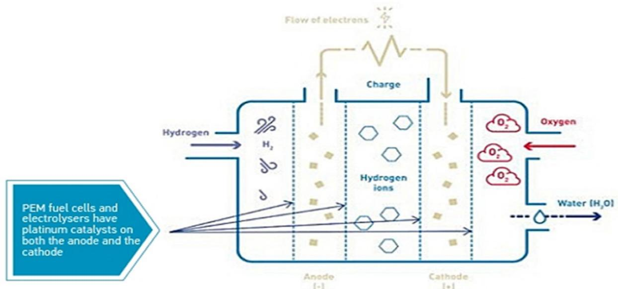
Source: Graphic from Airliquide Proton Exchange Membrane
