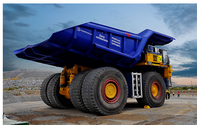
The world's largest hydrogen-powered mine haul truck designed to operate in everyday mining conditions. Picture credit: Anglo American plc. All rights reserved.
