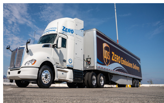
Toyota's FCEV truck combines the Kenworth T680 Class 8 model with its fuel cell electric technology
