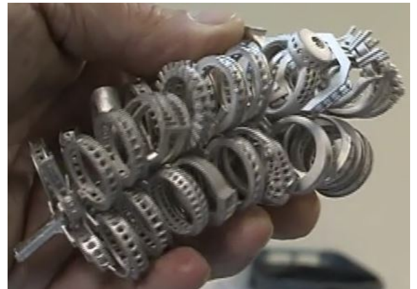
Platinum rings on a casting 'tree' - a mould that allows a number of rings to be cast at the same time
